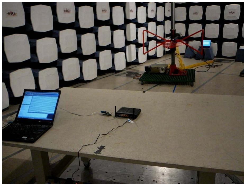
**14.5 Radiated Emissions – Front View (Above 1 GHz)**
