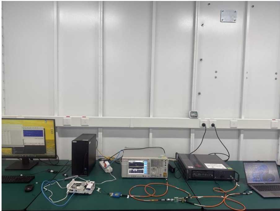
Description: DFS Test Setup - Mesh Mode
