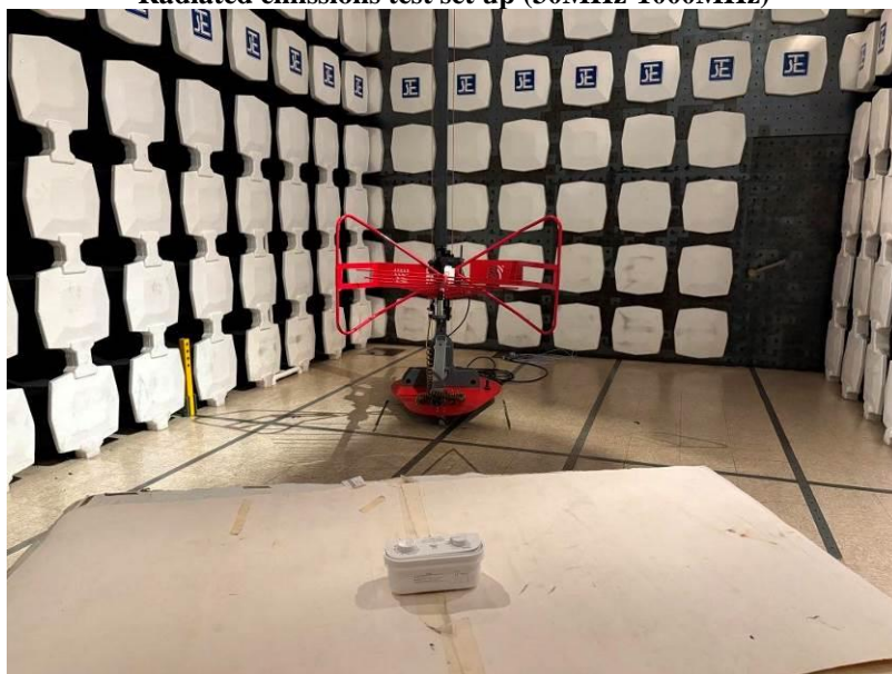
Radiated emissions test set up (30MHz-1000MHz)
