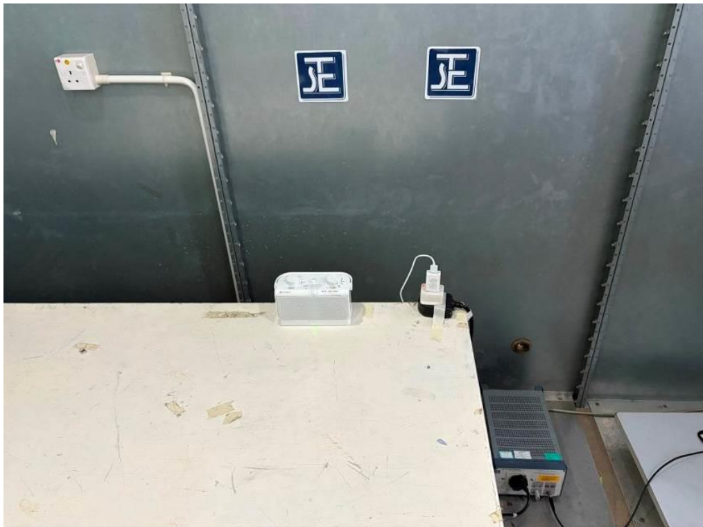
Measurement of Conducted Emission Test Set Up
