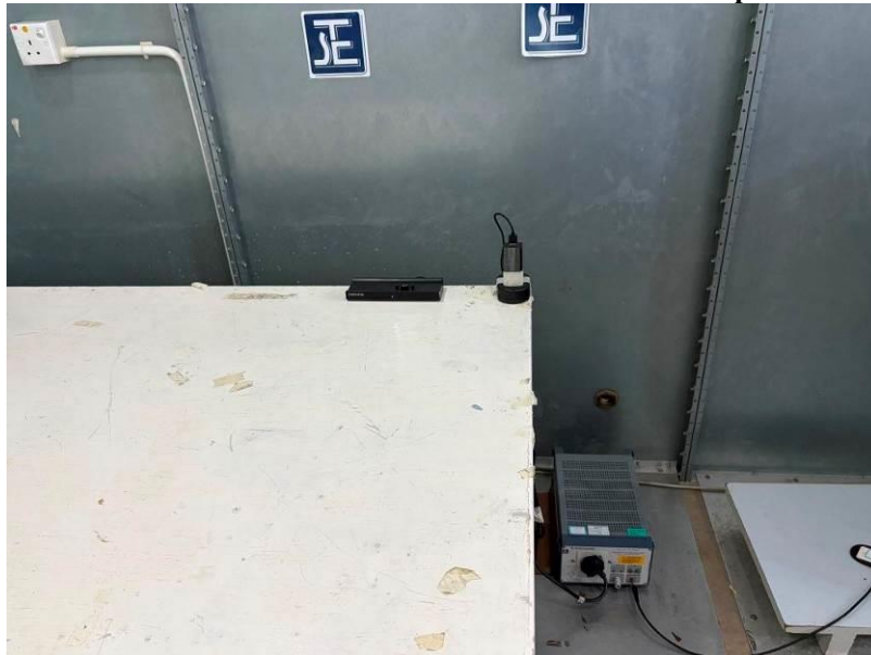
Measurement of Conducted Emission Test Set Up
