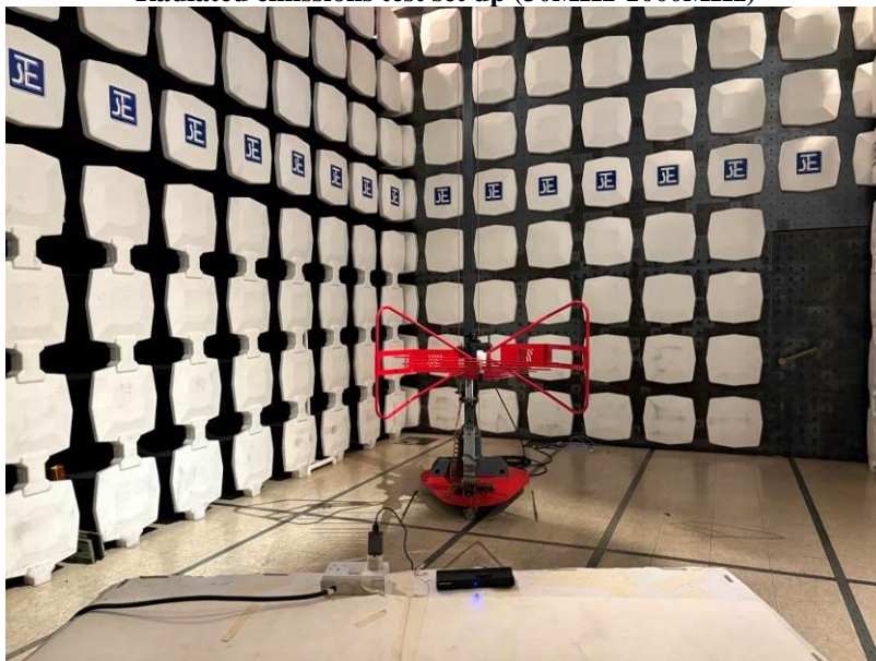
Radiated emissions test set up (30MHz-1000MHz)
