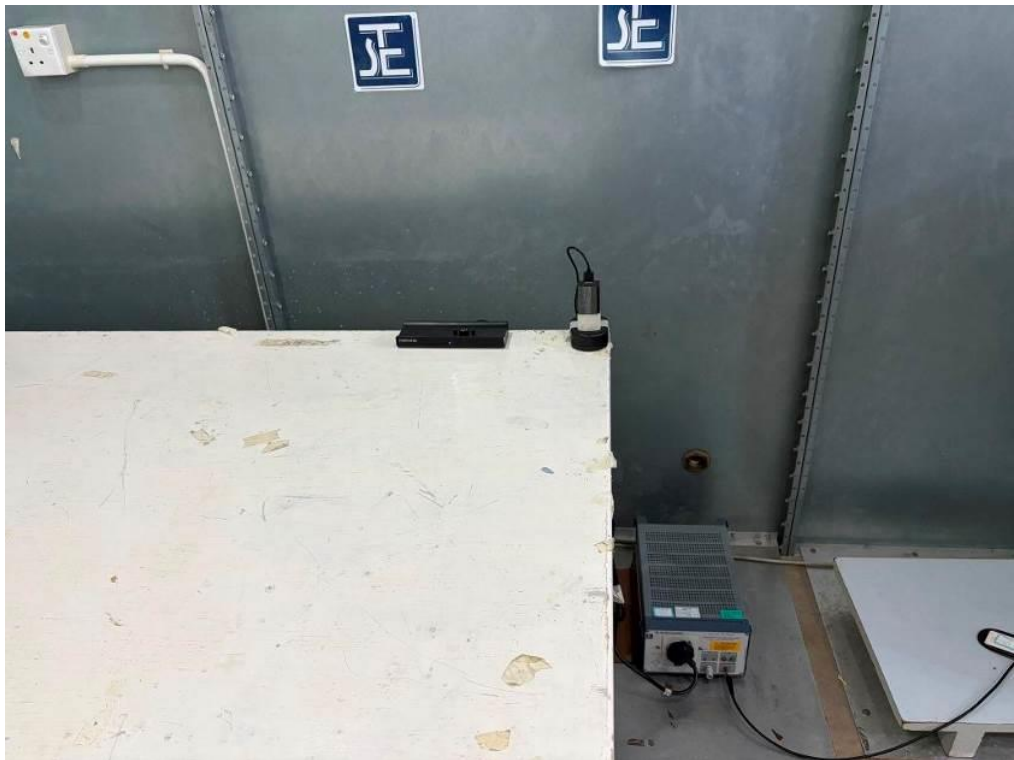
Measurement of Conducted Emission Test Set Up
