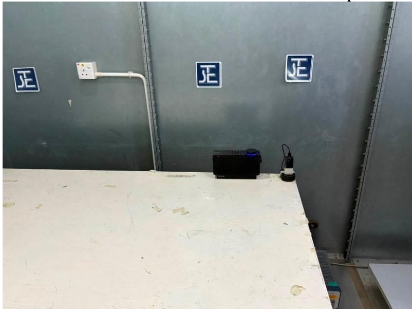
Measurement of Conducted Emission Test Set Up
