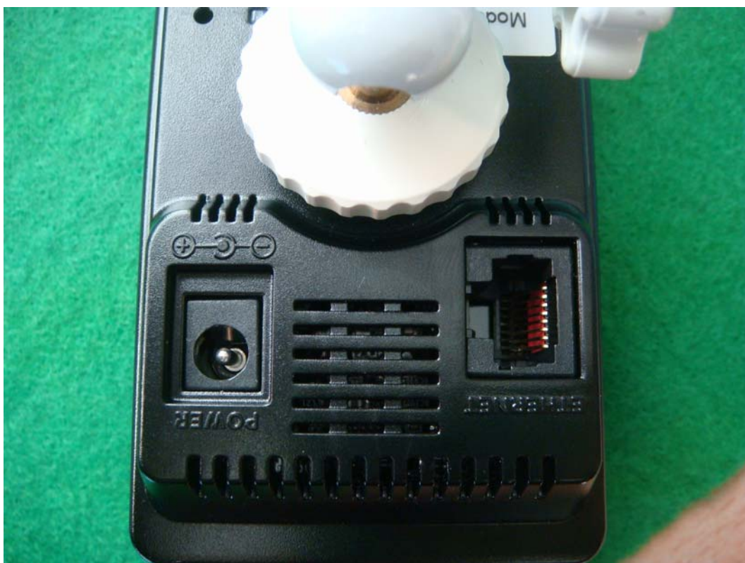
<Photograph 6: Interface View – DC input & Ethernet>
