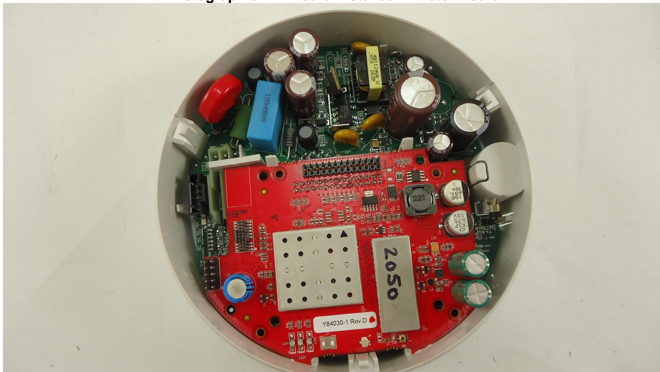
Photograph of RF Board Installed in Meter Board
