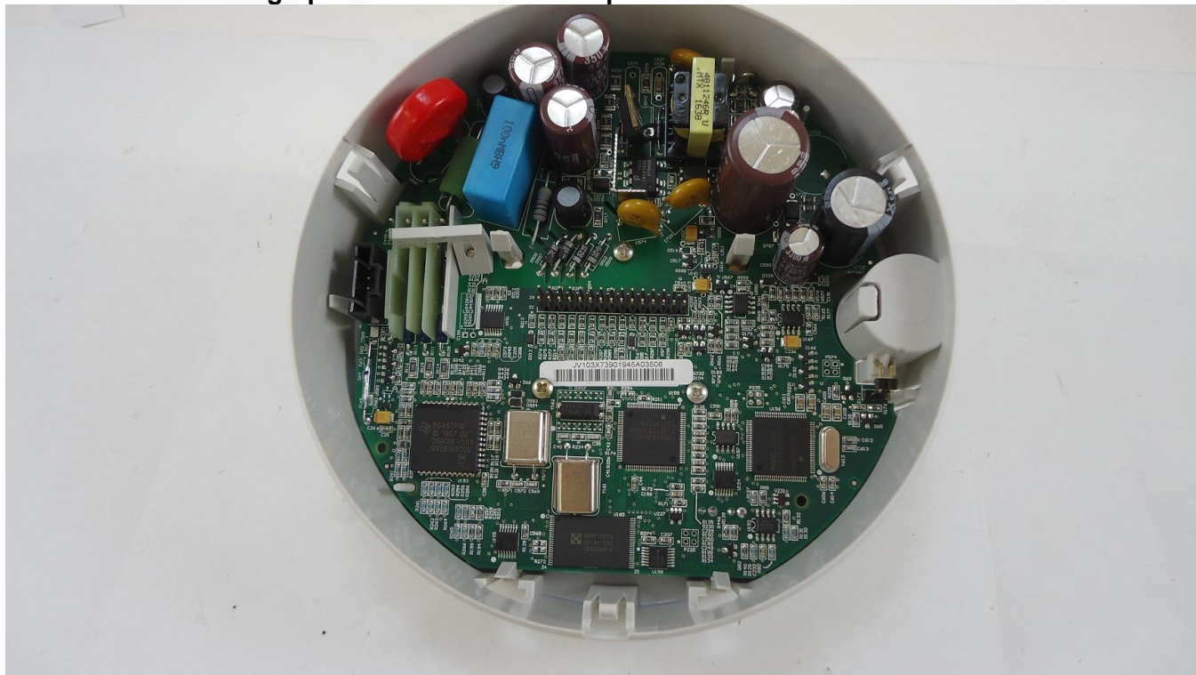
Photograph of Meter Board: Component side with shield removed
