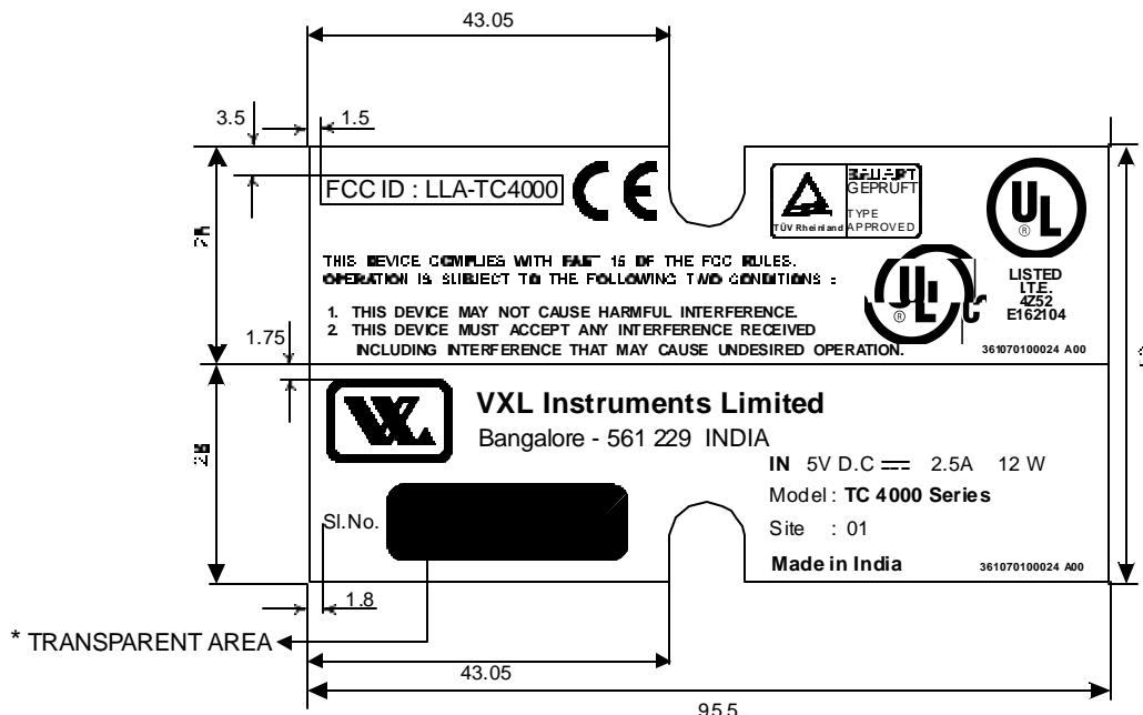
**MATERIAL** : POLY CARBONATE  $0.25^{+0.02}_{-0.00}$  THICK
