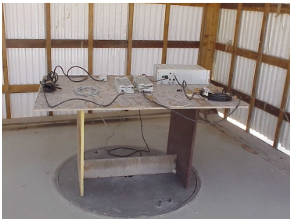
Photo # 5. Base Station + Subscriber Unit Radiated emission test on open site
