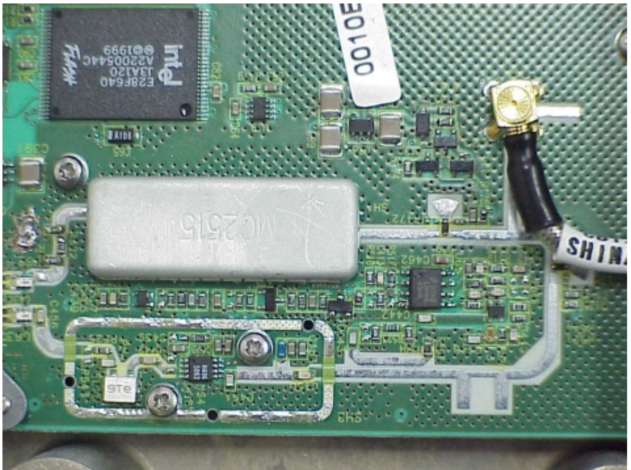
Photo 2 Radio Unit. Redesigned area (PWB component side)
