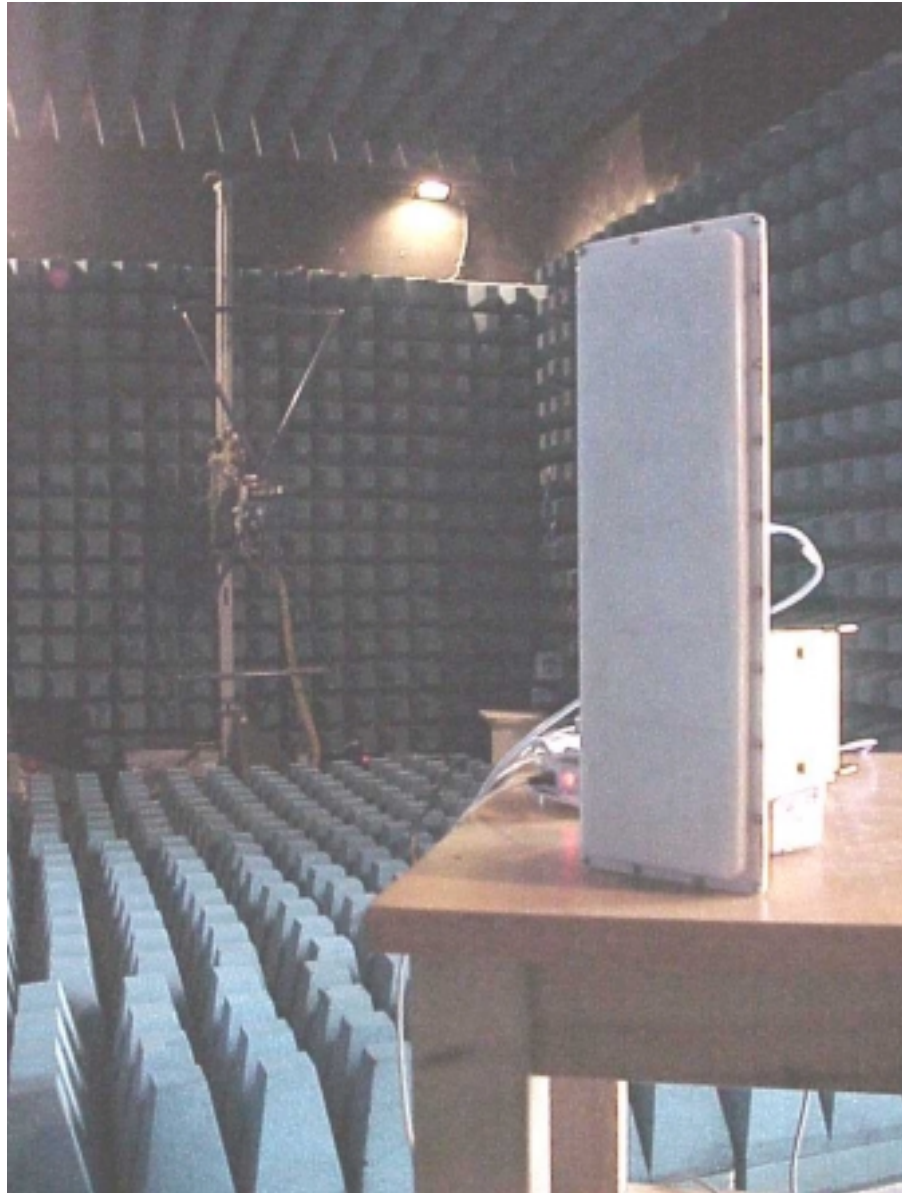
Photo #6. Radio unit with MTI sector antenna P/N MT-484025/NV. Spurious emission test
