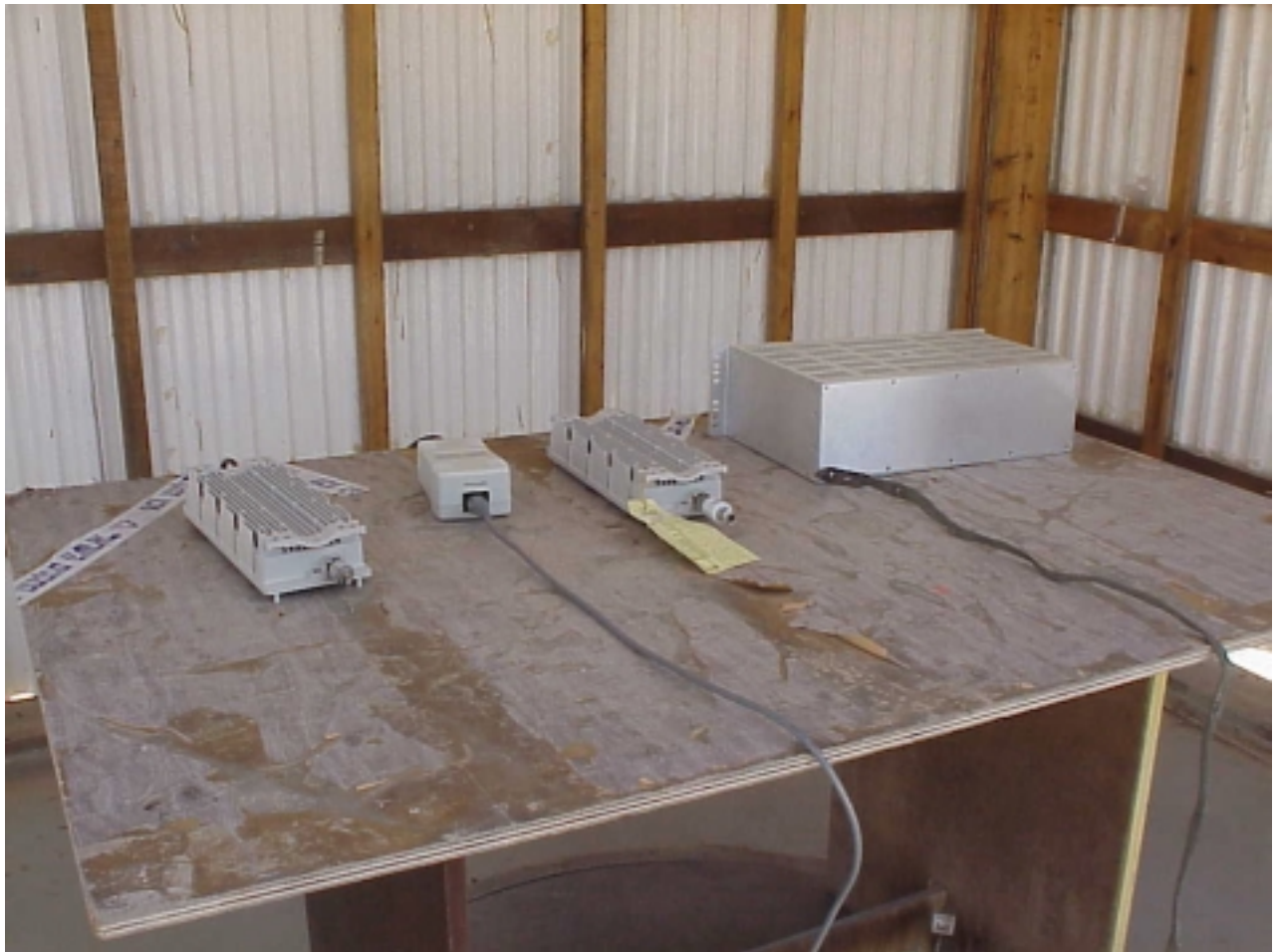
Photo #4. Base Station + Subscriber Unit Radiated emission test on open site
