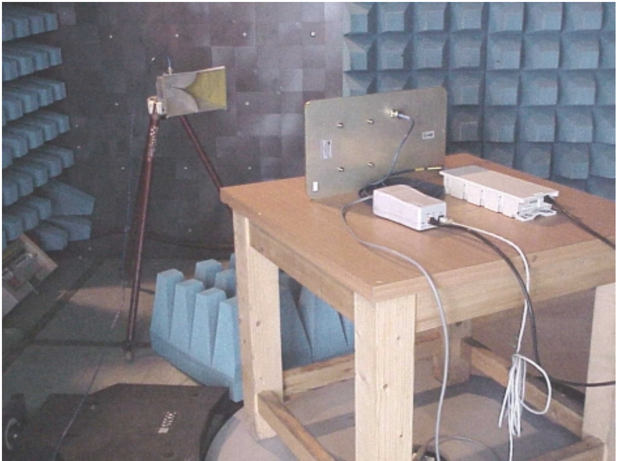
Photo #9 Spurious emissions test. Antenna .15-5.875 GHz P/N MT-484026/NV
