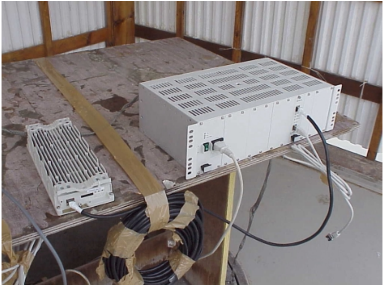
Photo #2. BreezeAccess VL System: Base Station Radiated emission test
