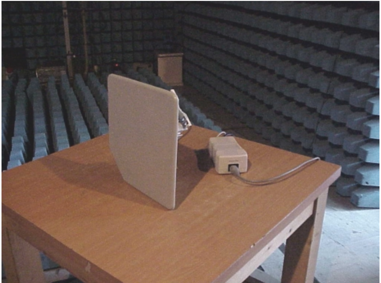
Photo #7 Spurious emission test, antenna MA-WA50-1X P/N AN1165 mfr Mars Antennas
