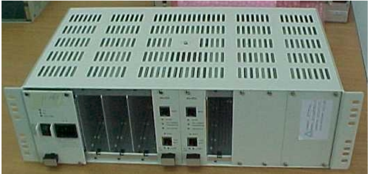
Photo # 12 AU-BS – Plugged-in indoor unit
