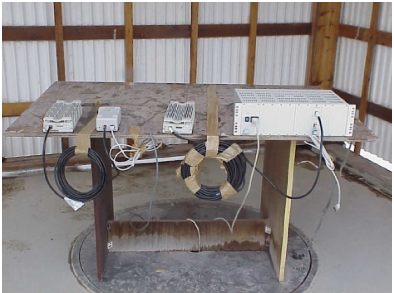
Photo #1. BreezeAccess VL System: Base Station + Subscriber Unit Radiated emission test
