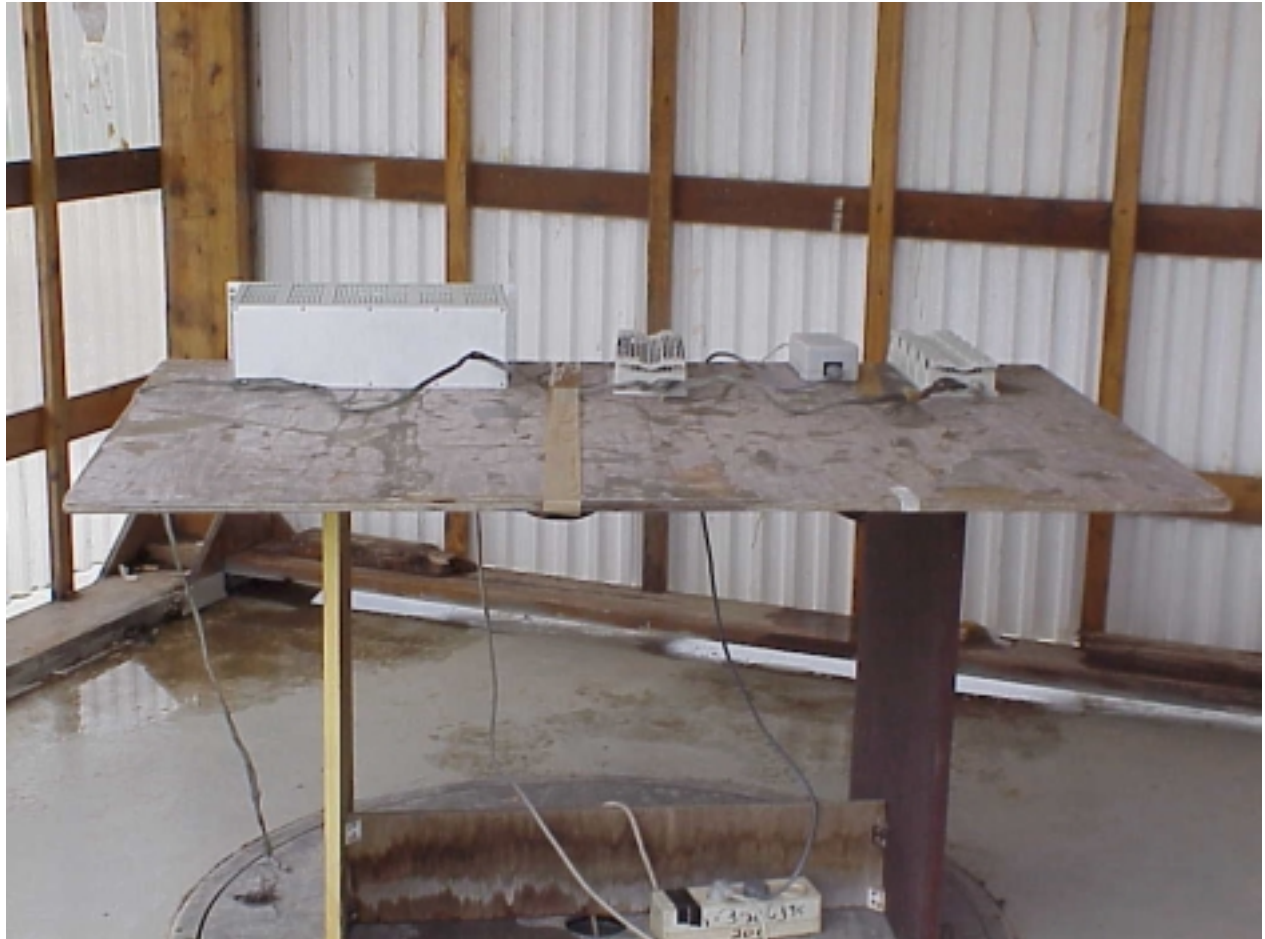
Photo #4. BreezeAccess VL System: Base Station + Subscriber Unit Radiated emission test
