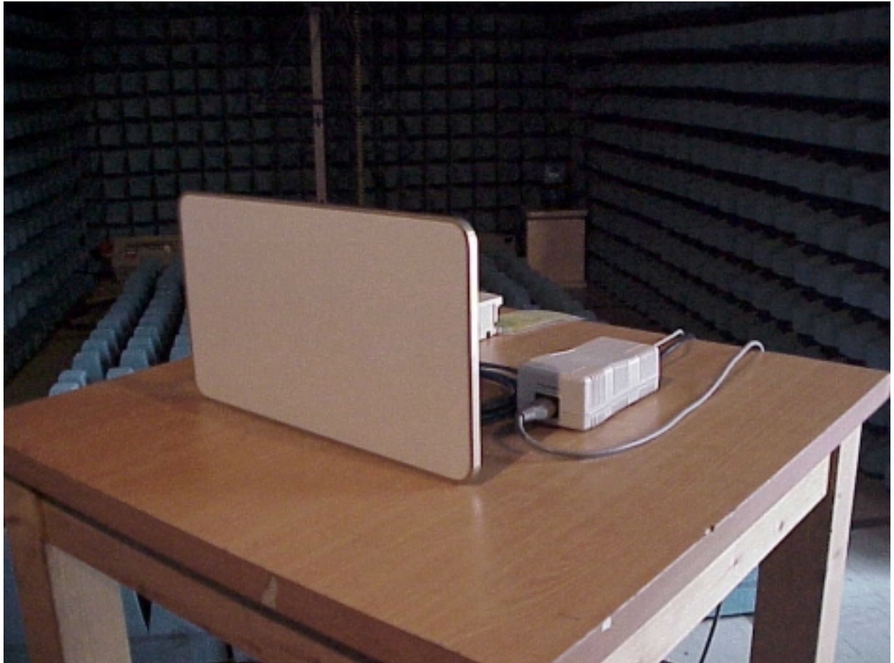
Photo #6 Spurious emissions test. Antenna 5.15-5.875 GHz P/N MT-484026/NV
