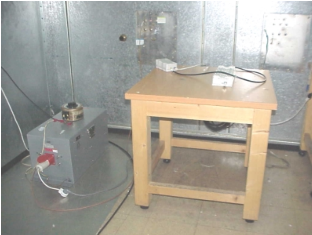
Photo #5. BreezeAccess VL System: Subscriber Unit Conducted emission test
