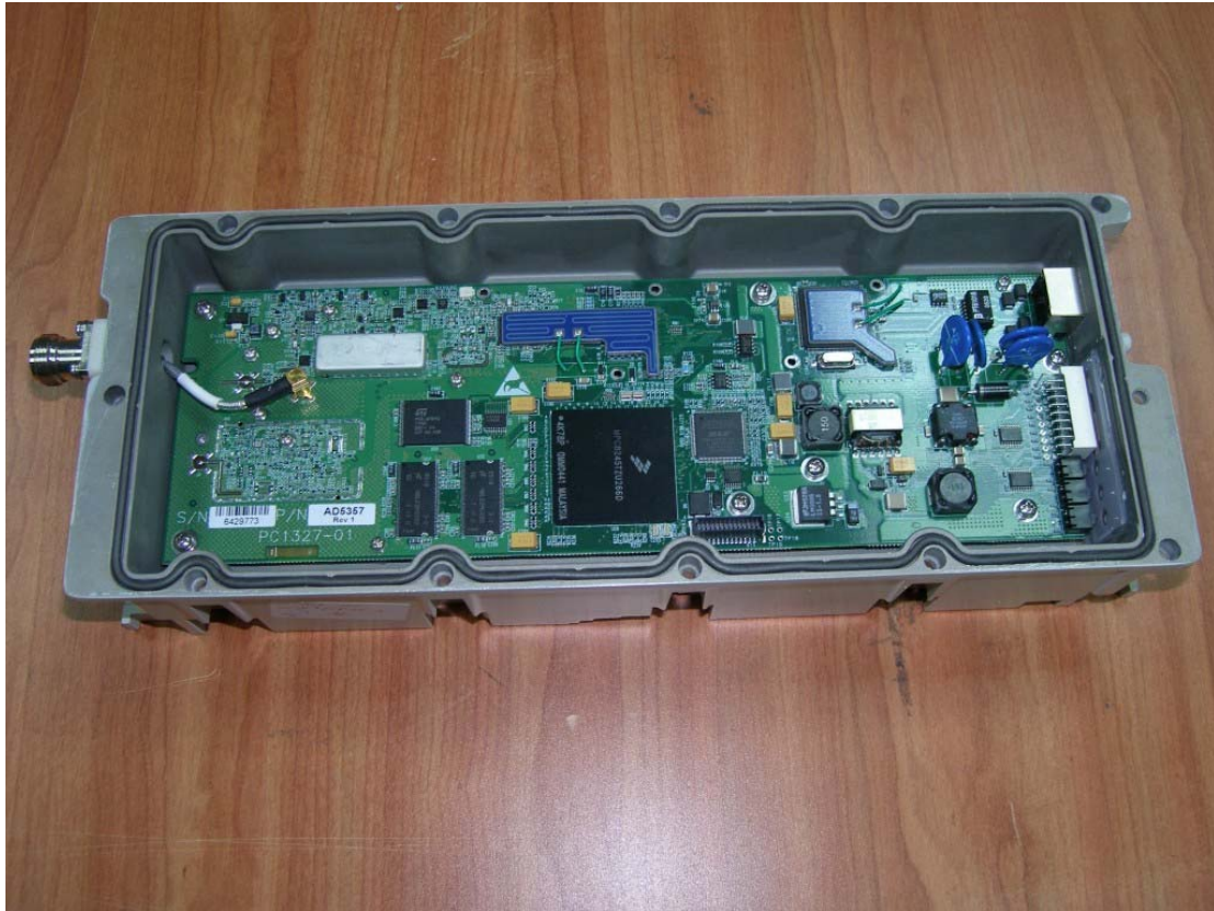
ODU , open cover PCB view
