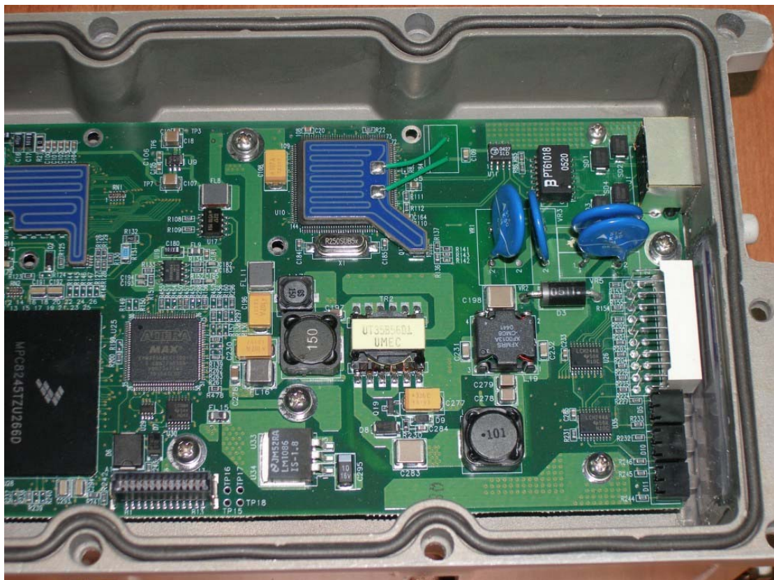
ODU components side , digital part
