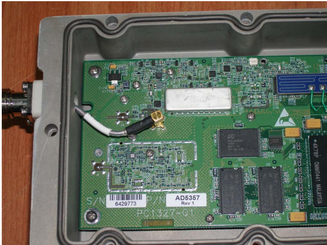
ODU components side
