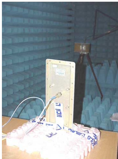
Photo # 5. P/N AN1152 Spurious emission test
