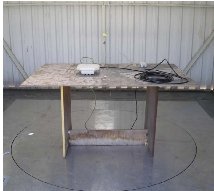
Photo 3. Radiated emissions test setup on OATS.
