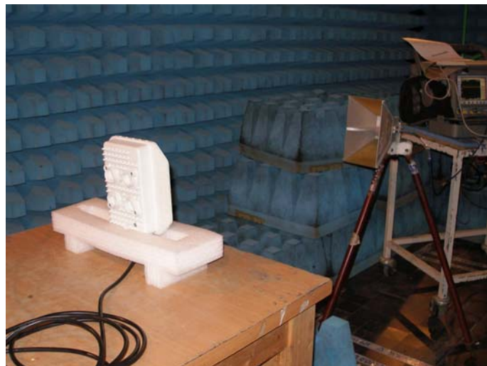
Photo #2. Radiated emissions test setup. Investigation test at 1m test distance.
