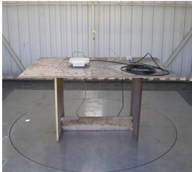
Photo #3. Radiated emissions test setup on OATS.
