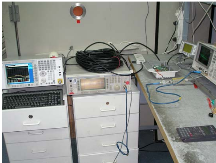
Photo #1. RF conducted emissions test setup.
