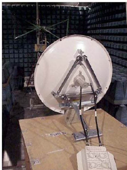
Photo #4. Test setup in anechoic chamber with parabolic antenna.
