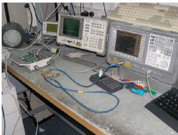
Photo #1. RF conducted emissions test setup.
