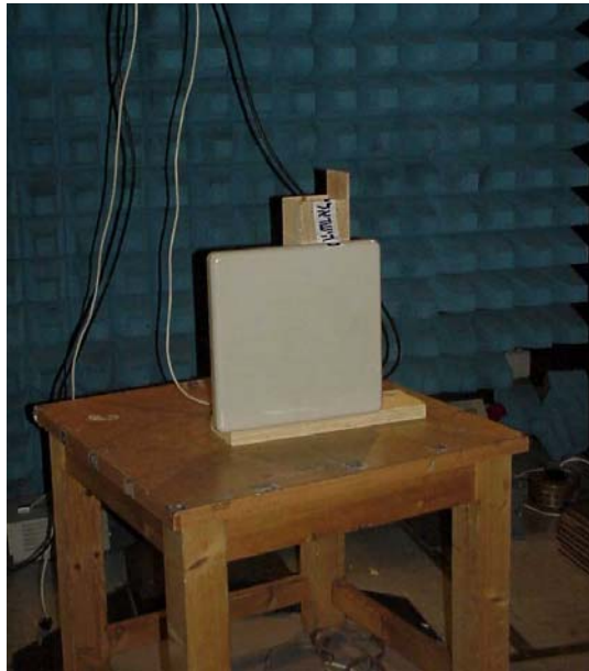
Photo #3. Test setup in anechoic chamber. Antenna Flat panel.
