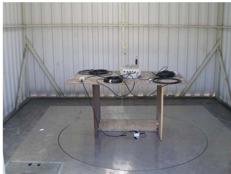
Photo #2. Radiated emissions test setup on OATS.
