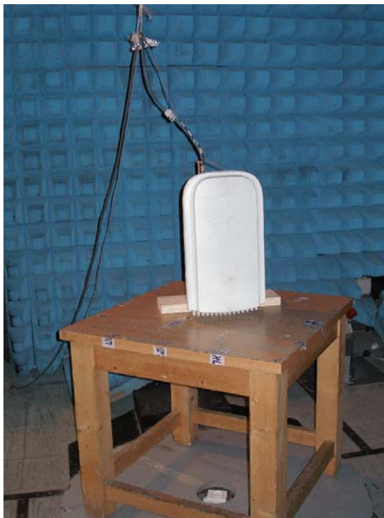
Photo 2. Test setup with internal antenna.
