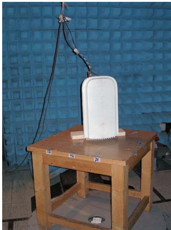
Photo 2. Test setup with internal antenna.
