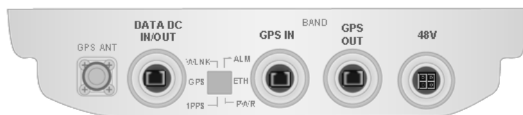
Figure 10: BTS Connections (Bottom View)
