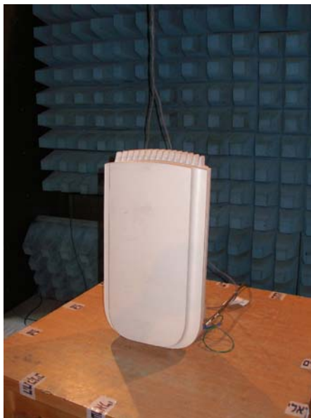
Photo 3. Investigation test setup with internal antenna.
