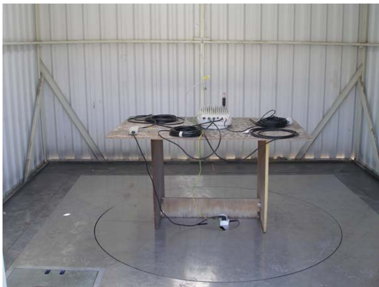
Photo 2. Test setup on OATS.
