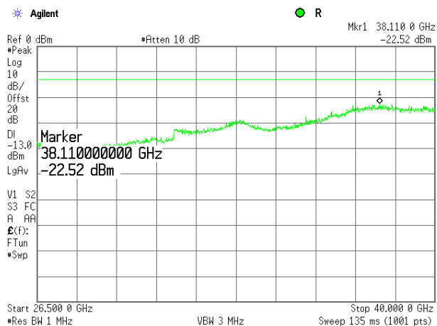
Plot 7.5.21 Spurious emission measurements in 26500 - 40000 MHz at high carrier frequency (Ant. 1)
