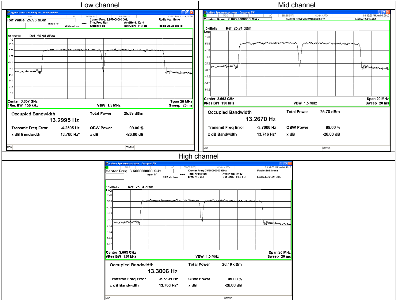
Plot 7.2.2 Occupied bandwidth test result, 14 MHz channel bandwidth
