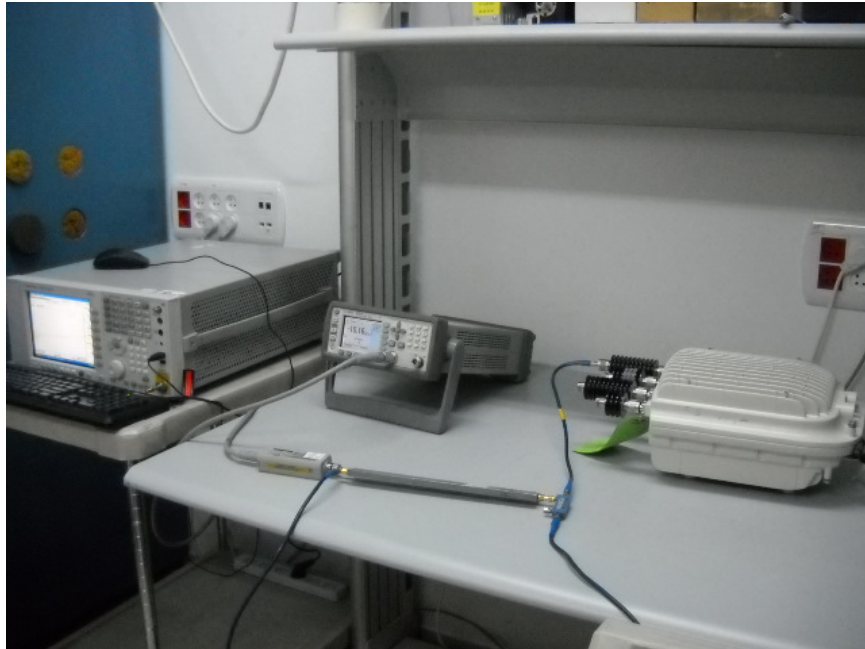
Photograph No.1 Peak output power measurement setup
