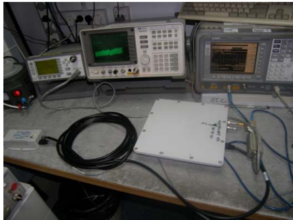
Photo #1. RF conducted emissions test setup.
