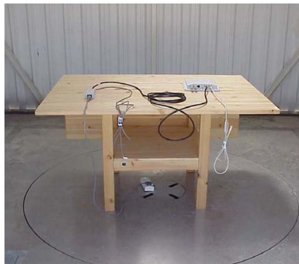
Photo #2. Radiated emissions test setup on OATS.
