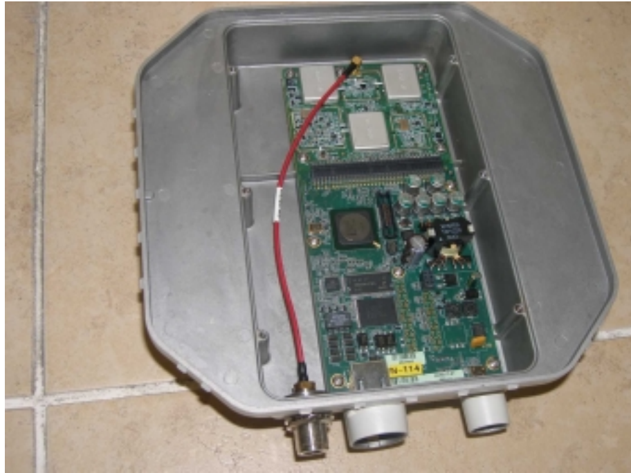
Photo 5. Outdoor unit. Internal view.
