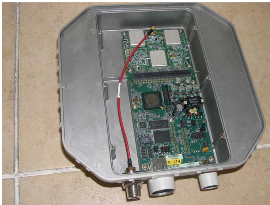
Photo 5. Outdoor unit. Internal view.
