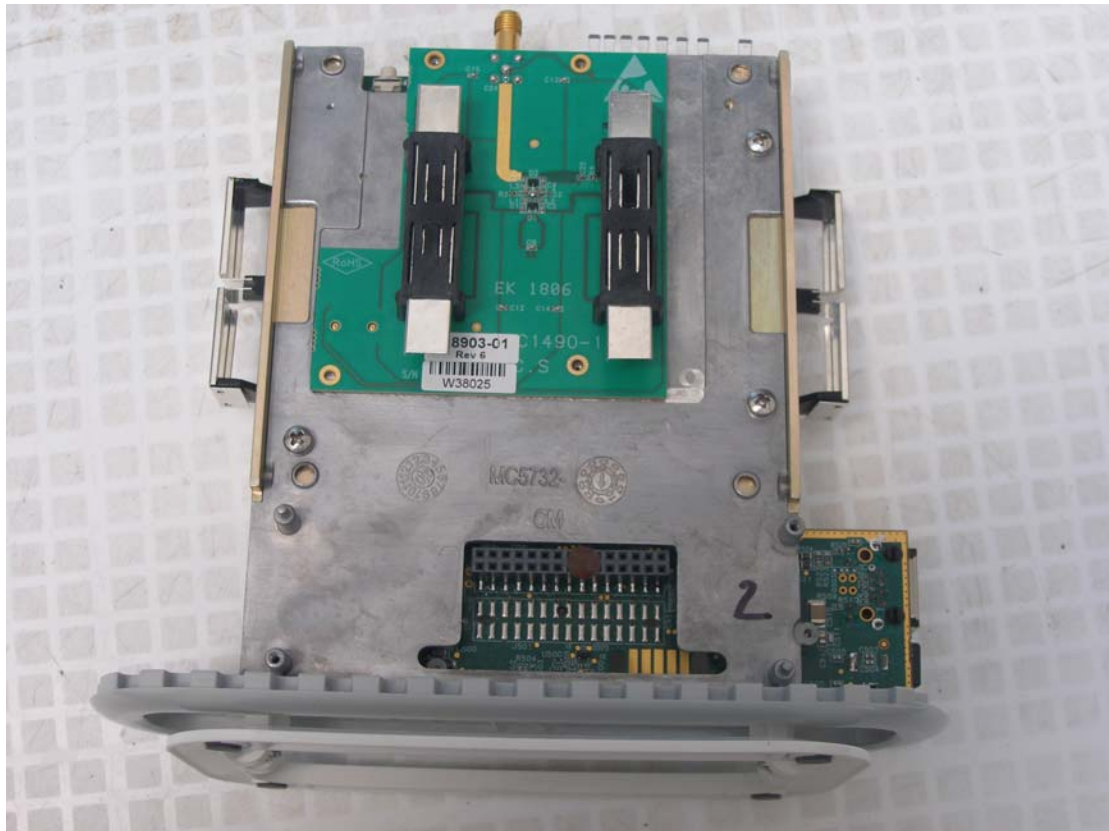
Photo9. CPE Si internal view, antennas
