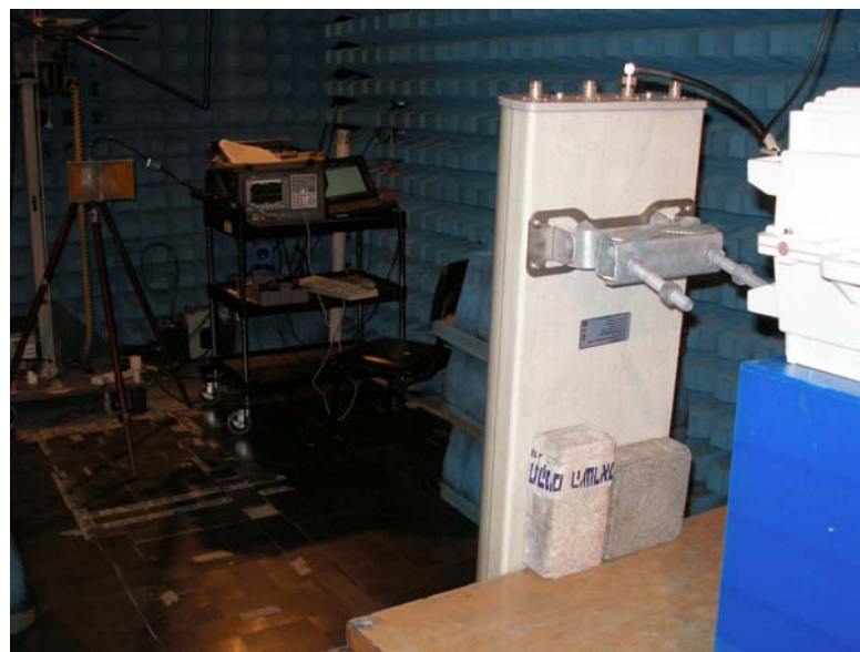
Photo 4. Test setup in anechoic chamber.
