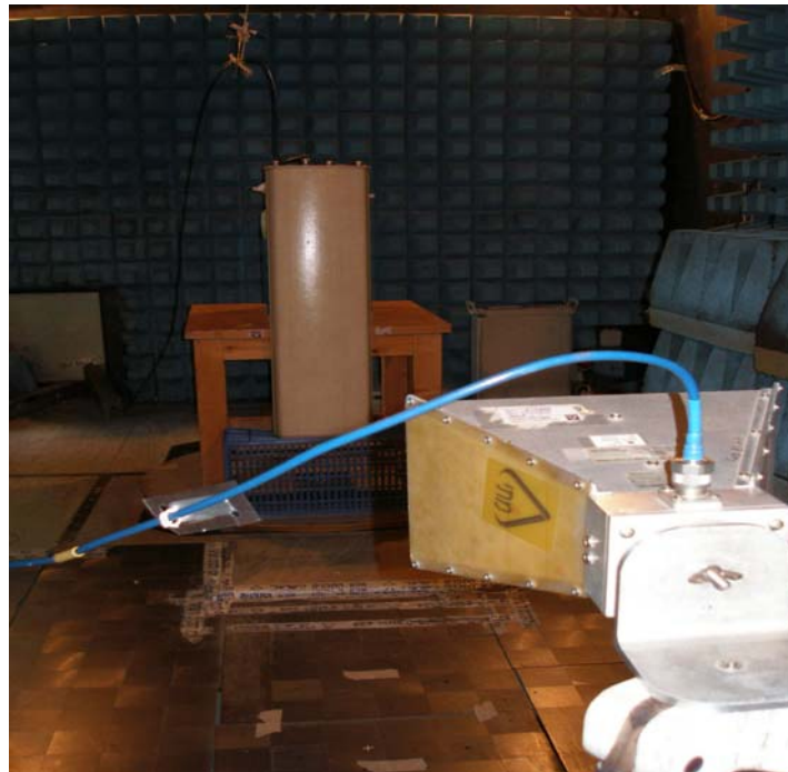
Photo 3. Test setup in anechoic chamber.
