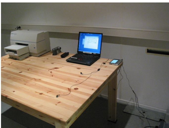
Picture 4 AC powerline conducted emission measurement Bluetooth TX / WLAN RX + Computer peripherals
