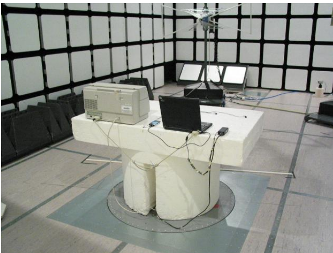
Picture 2. FCC Part 15B Radiated emissions
