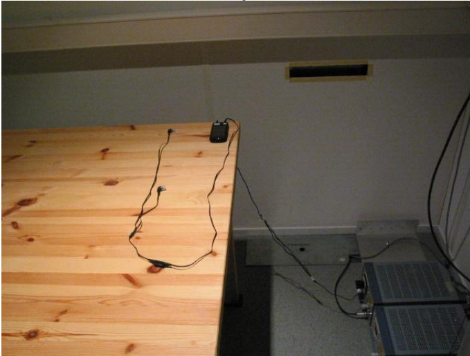
Picture 4. FCC Part 15B AC powerline conducted emissions (laptop)
