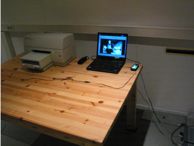
Picture 5. FCC Part 15B AC powerline conducted emissions (phone)
