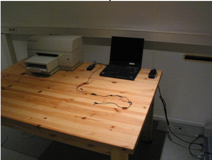
Picture 4. FCC Part 15B AC powerline conducted emissions (laptop)
