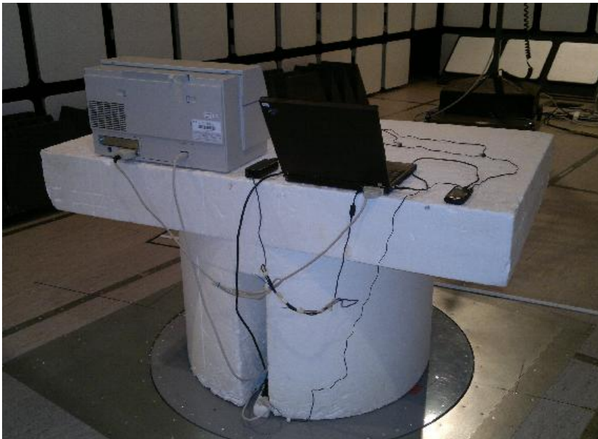
Picture 2. FCC Part 15B Radiated emissions
