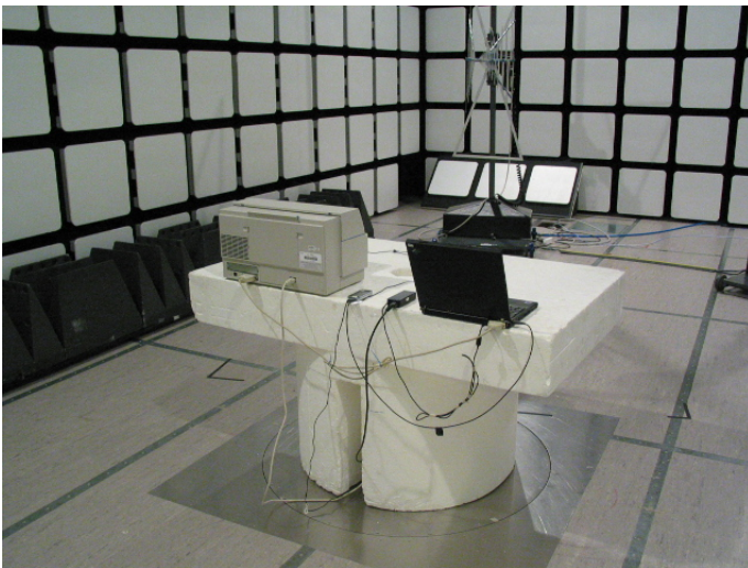
Picture 2 Radiated emission 15B
