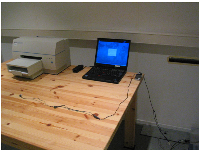
Picture 4 AC powerline conducted emission measurement 15B
