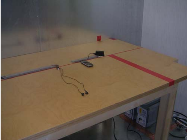
Picture 3 AC powerline conducted emission measurement 15C
