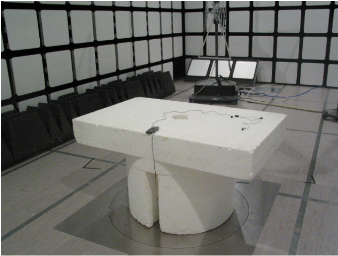
Picture 3 Radiated emission measurement GSM RX + GPS receiver on / FM radio on
