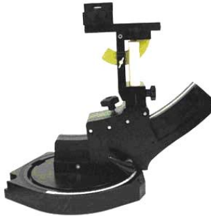
Device holder supplied by SPEAG
