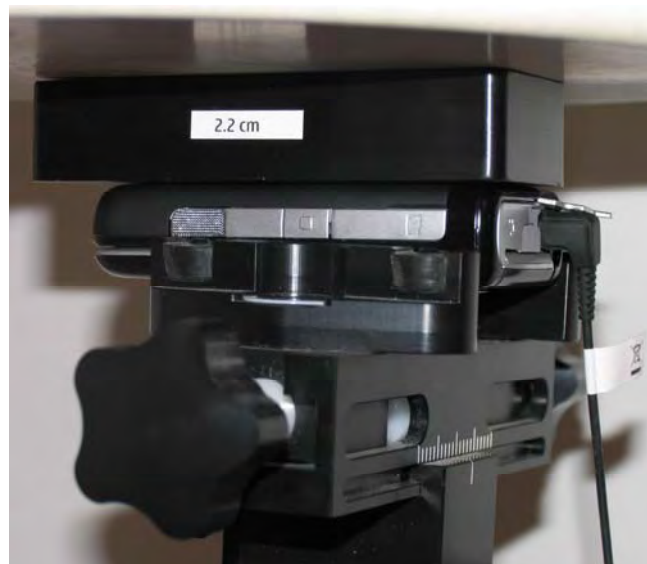
Photo of the device positioned for Body SAR measurement. The spacer was removed for the tests.
