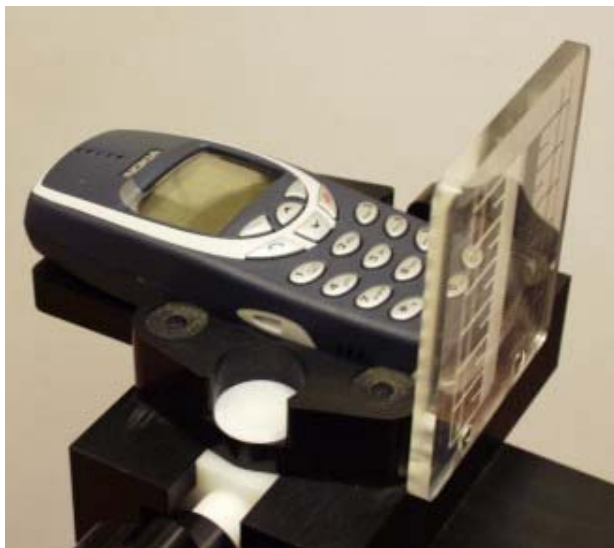
Figure 2. Positioning of the phone
