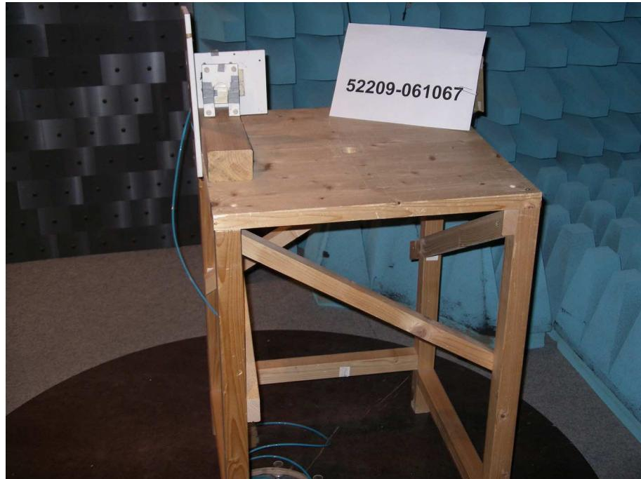
**Test setup for radiated emission measurement
