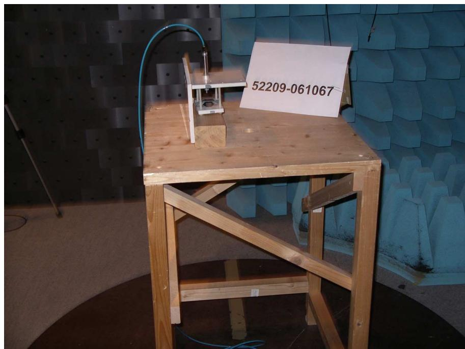
**Test setup for radiated emission measurement
