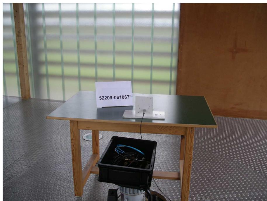
**Test setup for radiated emission measurement
