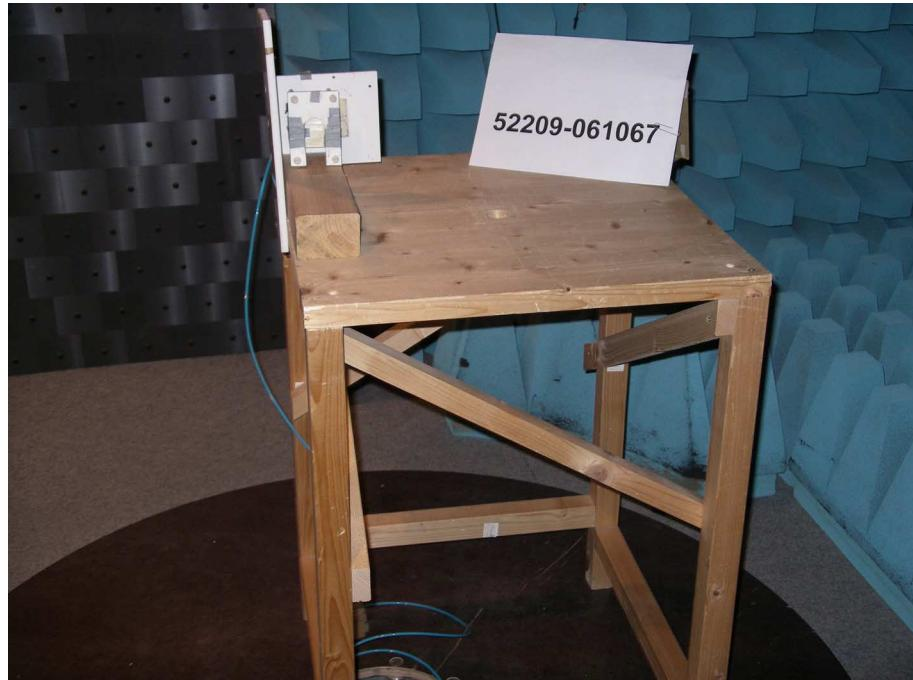
**Test setup for radiated emission measurement
