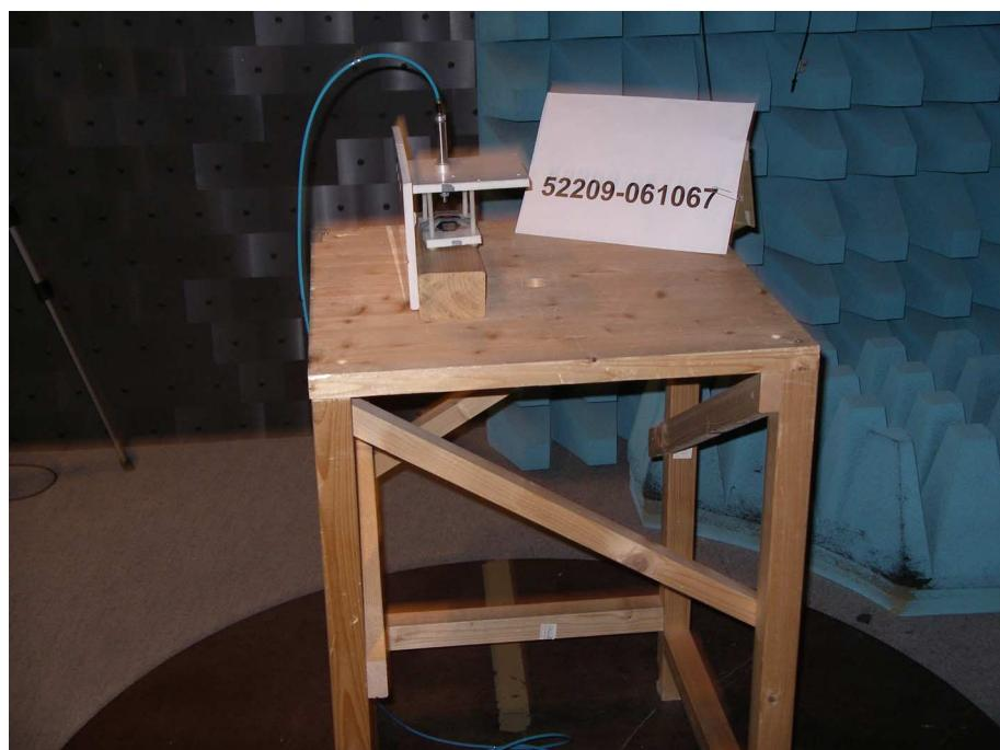
**Test setup for radiated emission measurement
