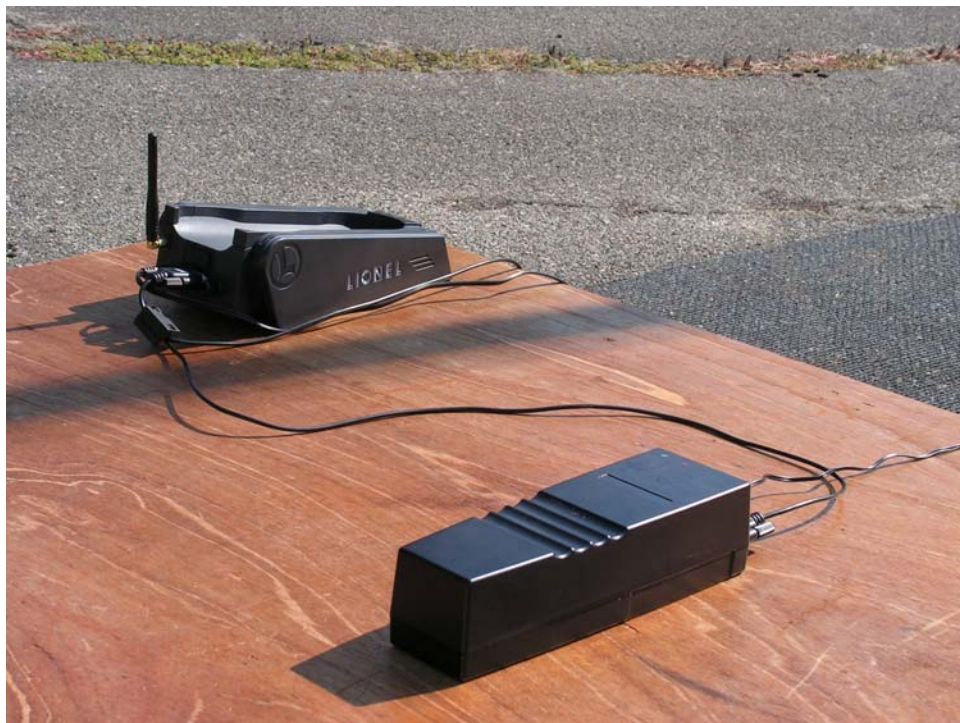
DUT on OATS (close-up) – one of three antenna axes tested
