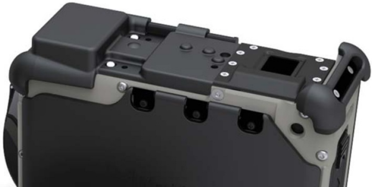
Figure 3: Assembled View (BPAC Host Antenna Overmold)
