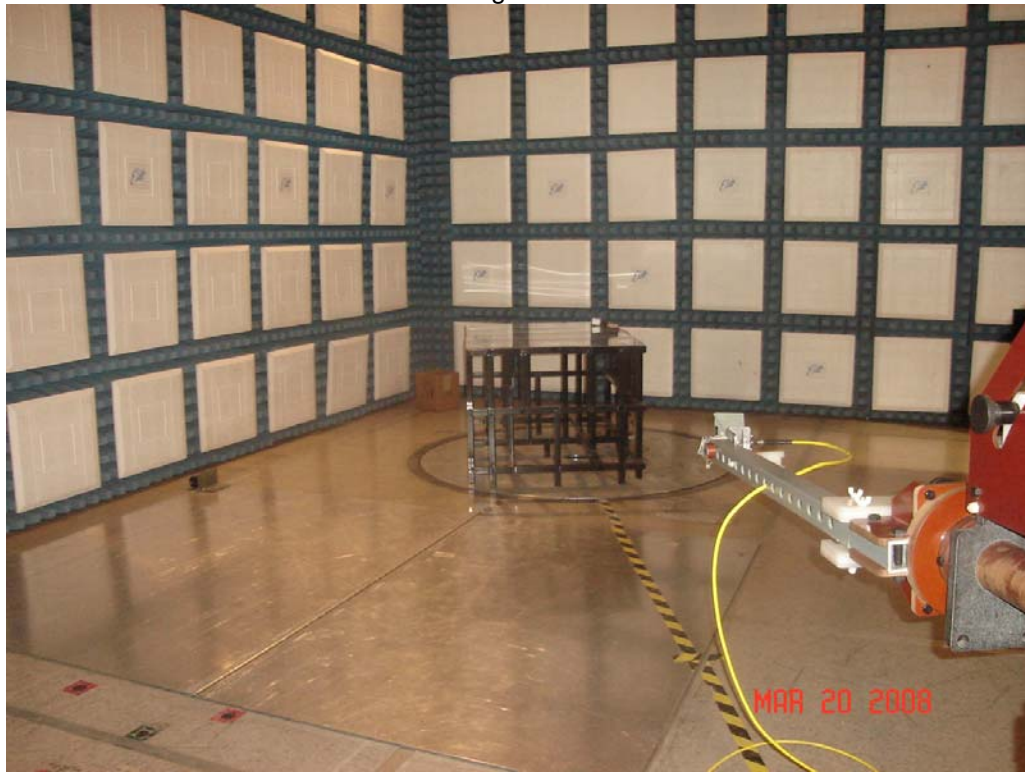
Test Set-up for Radiated Emissions – Horizontal Polarization
