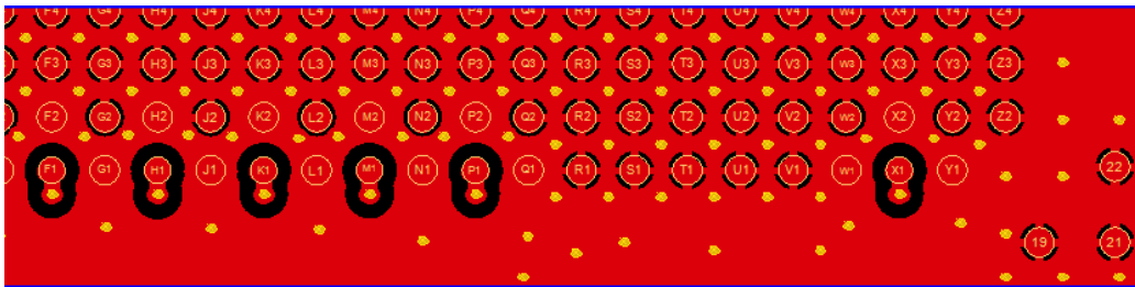
Figure 9-3: Antenna Pad Ground Cutout Recommended (Main Board, top layer/NAD side)
