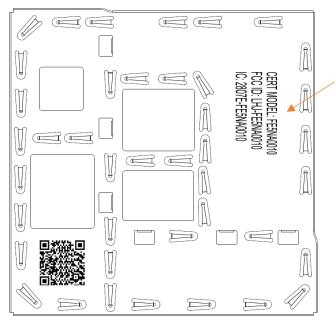
Laser etching on top of the shield the Model Name and Regulatory Markings.
